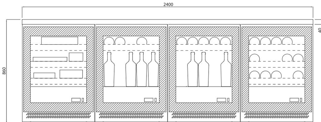
CANALISATION DE VITRES MOD "HAVANA" H=1260mm AVEC PORTES BATTANTES DROIT / GAUCHE ÉQUIPÉES D'UNE POUR VINS TEMPERATURE (+10/+18°C) AVEC UN TIROIR ET PLAN INTERMÉDIAIRE / DE FOND POUR METTRE LES BOUTEILLES VERTICALEMENT ET MEUBLES EN CUIR LAQUÉ.
