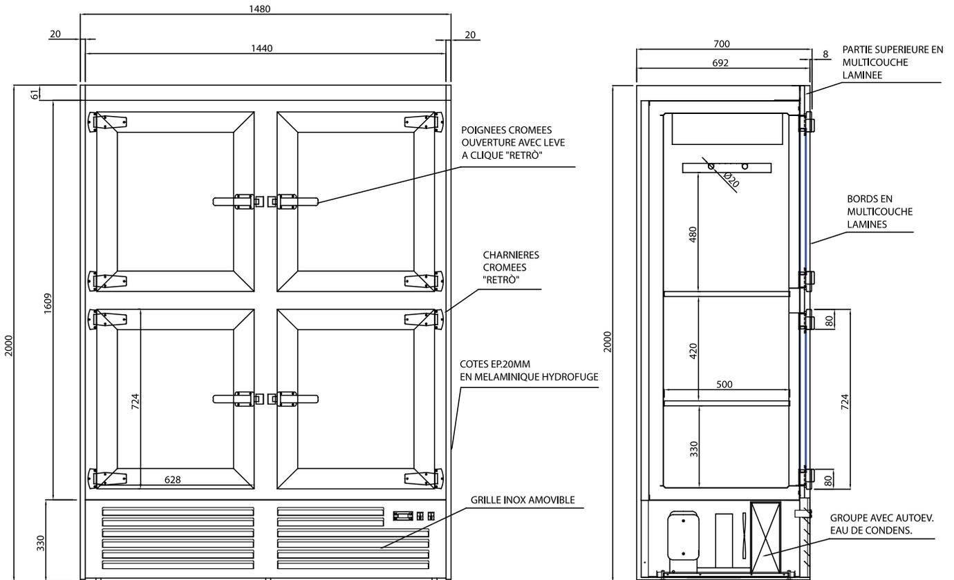
ELEMENT L=1480\*700\*H=2000 mm AVEC COQUE ISOLEE, AVEC POLYURETHANE ECOLOGIQUE EN FAIBLE DENSITE, INTERIEUR EN INOX AISI 304, SYSTEME A DETENTEUR R134A VENTILE, ECLAIRAGE LED VERTICAL PLACE DU SUPPORT CENTRALE, SOUBASSEMENT H=330 mm, AVEC GRILLE INOX SCOTCH-BRITE ET GROUPE CONNECTE A L'INTERIEUR OU DISTANT. ALIMENTATION ELECTRIQUE 220V/50HZ/1, PUISSANCE ABSORBE P=420W,CAPACITE INTERNE TOTALE 120 lt, T°+4/8°C
