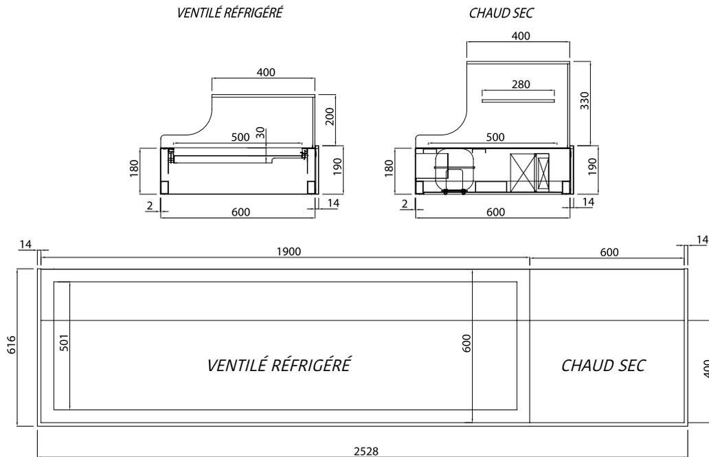
ÉLÉMENT PLUG-IN AVEC INSTALLATION À CAPILLAIRE R290 OU R134A, AVEC THERMOSTATS DIGITAUX TOUCH-SCREEN, AVEC CHALEUR DISSIPÉE PAR LE CONDENSEUR RÉCUPÉRÉ DANS LE PLAN CHAUD, SPÉCIALEMENT CONÇU POUR ÊTRE POSÉ SUR DES COMPTOIRS DE BAR EXISTANTS (OU SUR DES MODULES DE RÉFRIGÉRATION) SANS AVOIR À EFFECTUER DES TRAVAUX COMPLIQUÉS DE MONTAGE (IL SUFFIT DE FIXER COMME INDiqué DANS LE SCHÉMA CI-DESSOUS).
