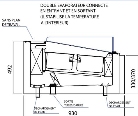
DOUBLE EVAPORATEUR CONNECTE EN ENTRANT ET EN SORTANT (IL STABILISE LA TEMPERATURE A L'INTERIEUR)
